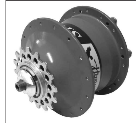
Rohloff SPEEDHUB 500/14 CC (snelspanas)
